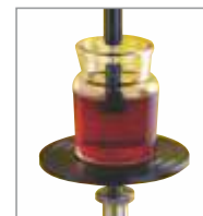
DETERMINATION OF GELATIN BLOOM STRENGTH
